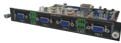
D6104VC 4 Channels VGA Digital Output Card
