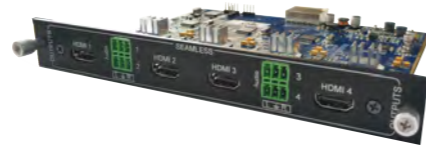
D6104HC 4 Channels HDMI Digital Output Card
