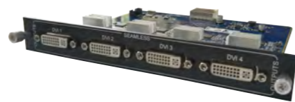
D6104DC 4 Channels DVI Digital Output Card
